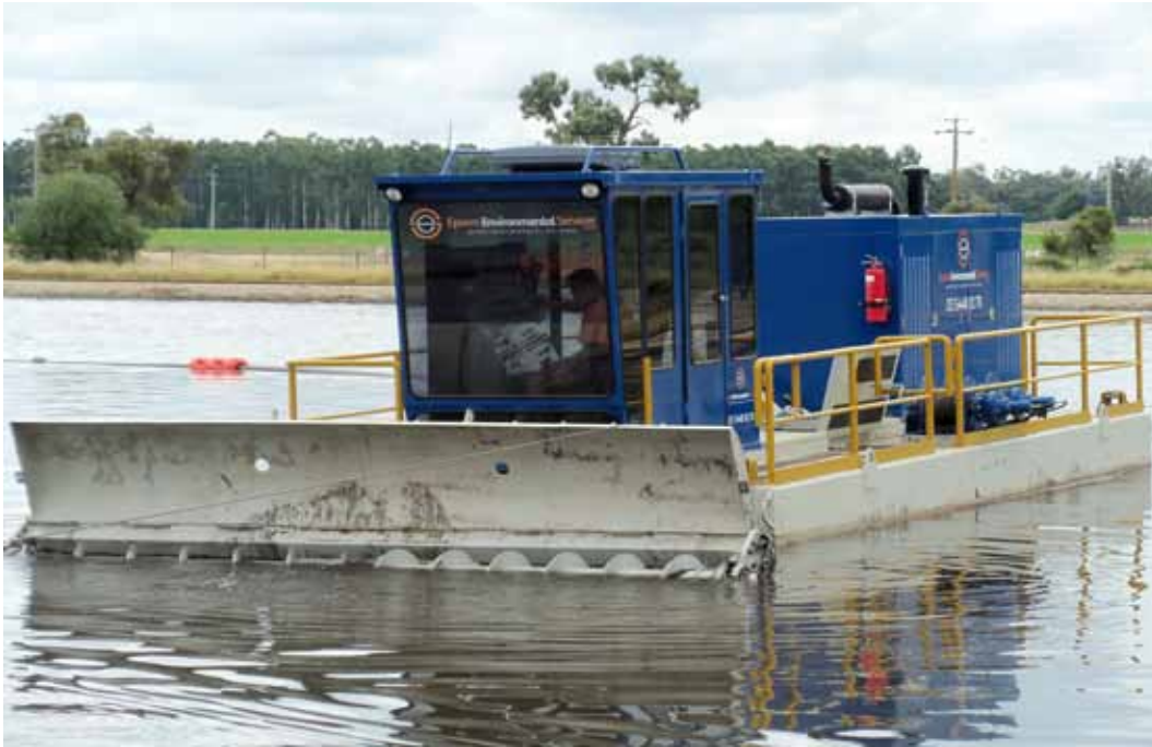
FIGURE 4.4 SLUDGE SUCTION DREDGE BARGE
