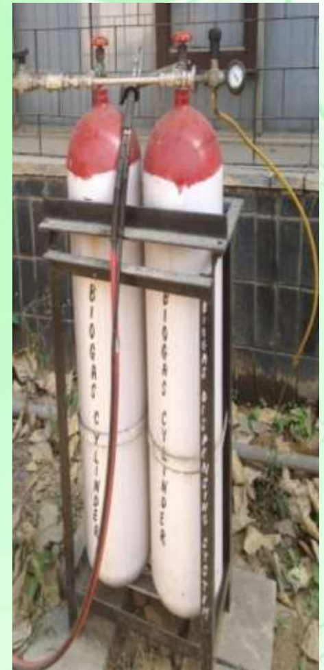
Two cylinder cascade for bottling of upgraded biogas
