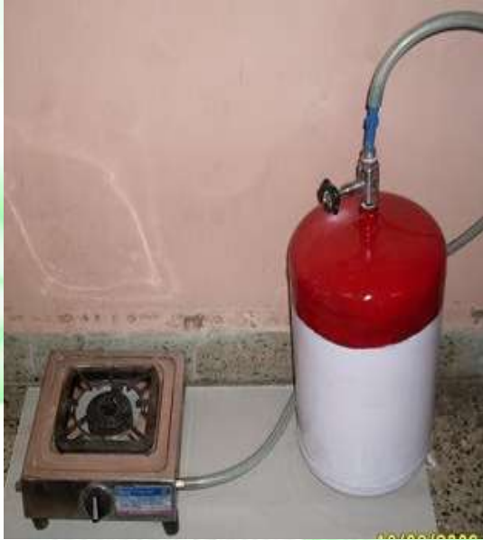
Upgraded and bottled biogas for use as a cooking fuel
