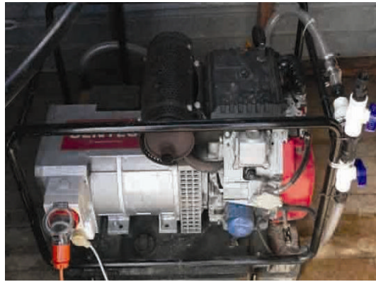
Petrol powered electricity generator converted to biogas
