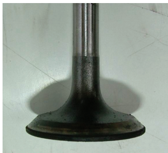
Fig. 2. Carbon deposits on main engine components before and after 3500 hours durability test
