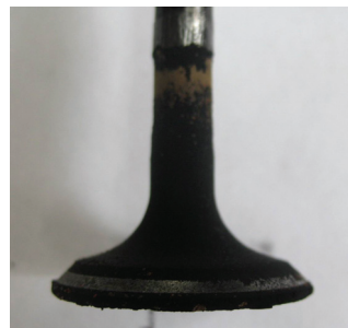
Fig. 2. Carbon deposits on main engine components before and after 3500 hours durability test
